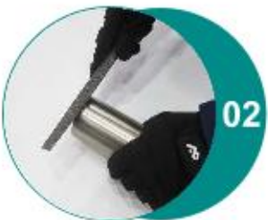
Deburr and chamfer the pipe end.
