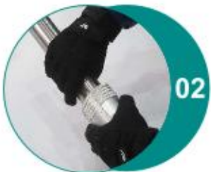
Deburr and chamfer the pipe end.
